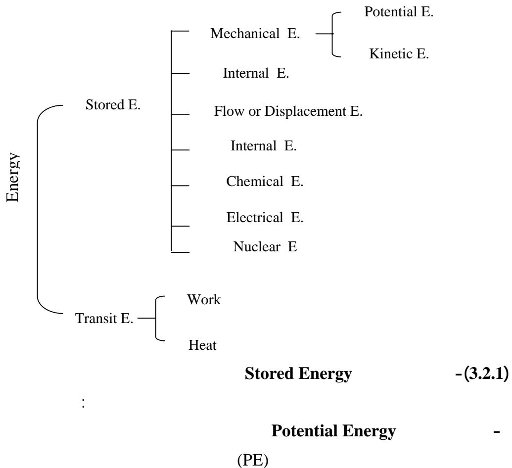
$$PE = F \times Z = m \times g \times z \quad \dots\dots (3.1)$$
