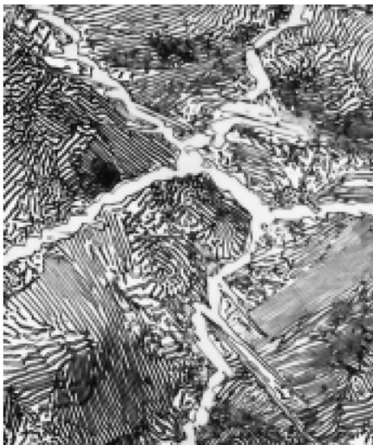
FIGURE 10.35 Photomicrograph of a 1.4 wt% C steel having a microstructure consisting of a white proeutectoid cementite network surrounding the pearlite colonies. 1000 \times . (Copyright 1971 by United States Steel Corporation.)
