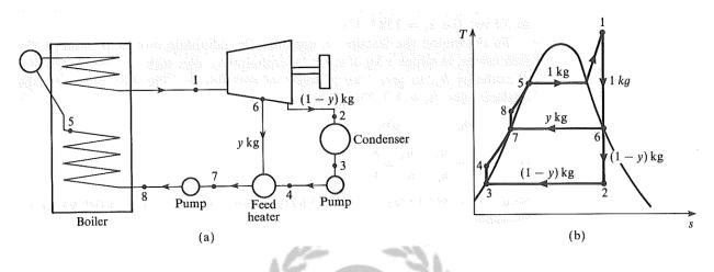
the amount of extracted steam can be determined by energy balance around the heater;
