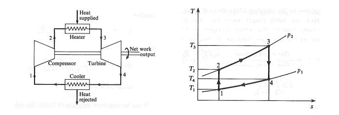
The steady-flow energy equation will have the following form in analysis and each process is to be considered in turn;
