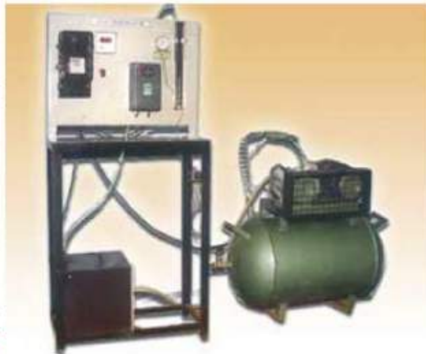
Measuring efficiency of compressor.
