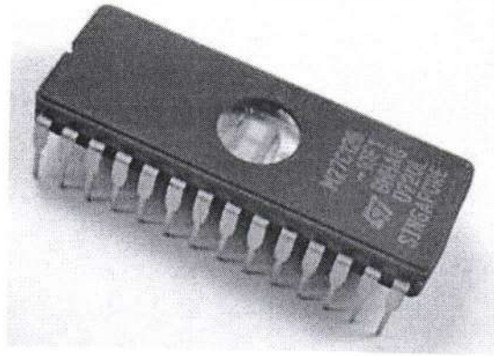
Figure 3.3: Erasable Programmable Read Only Memory (EPROM)
