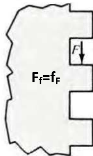
(a) Force normal to a square thread
