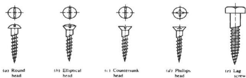
FIGURE 18-4 Sheet-metal and lag screws (R. P. Hoelscher et al., Graphics for Engineers , New York: John Wiley & Sons, 1968)
