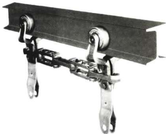
(b) Chain and roller system supported on an I-beam
