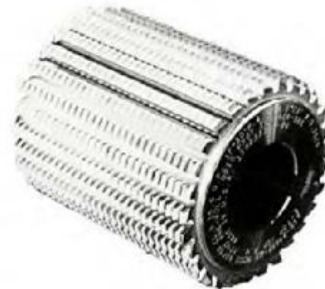
(d) Hob for high pitch gears having small teeth
