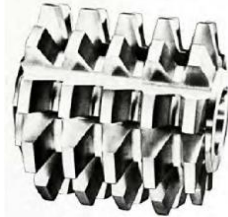
(c) Hob for small pitch gears having large teeth
