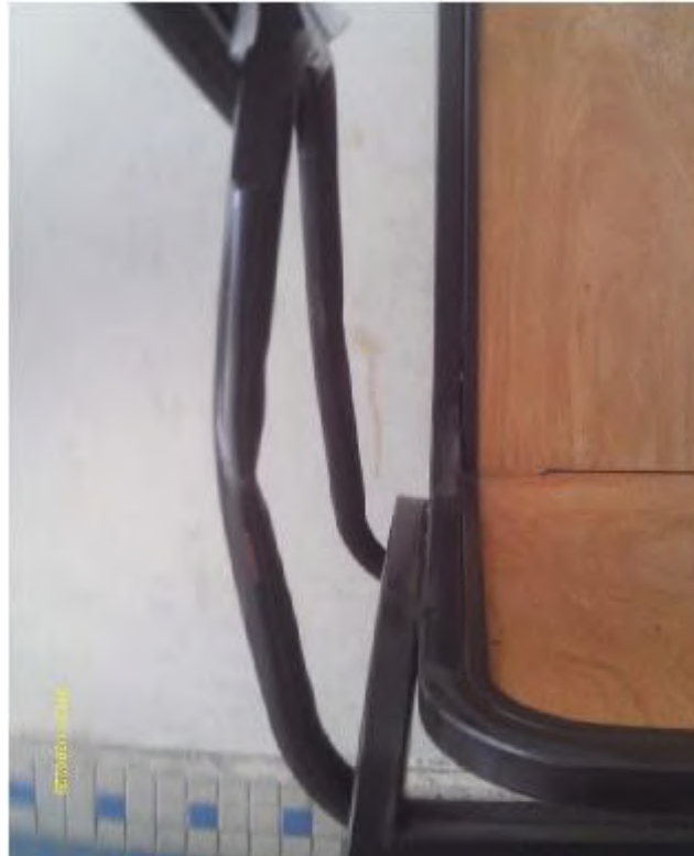
Bending of holding frame
