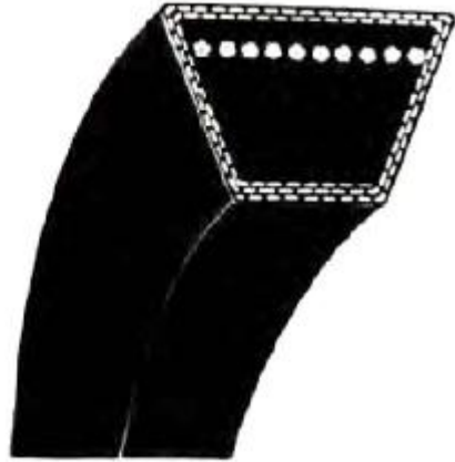
(a) Wrapped construction
