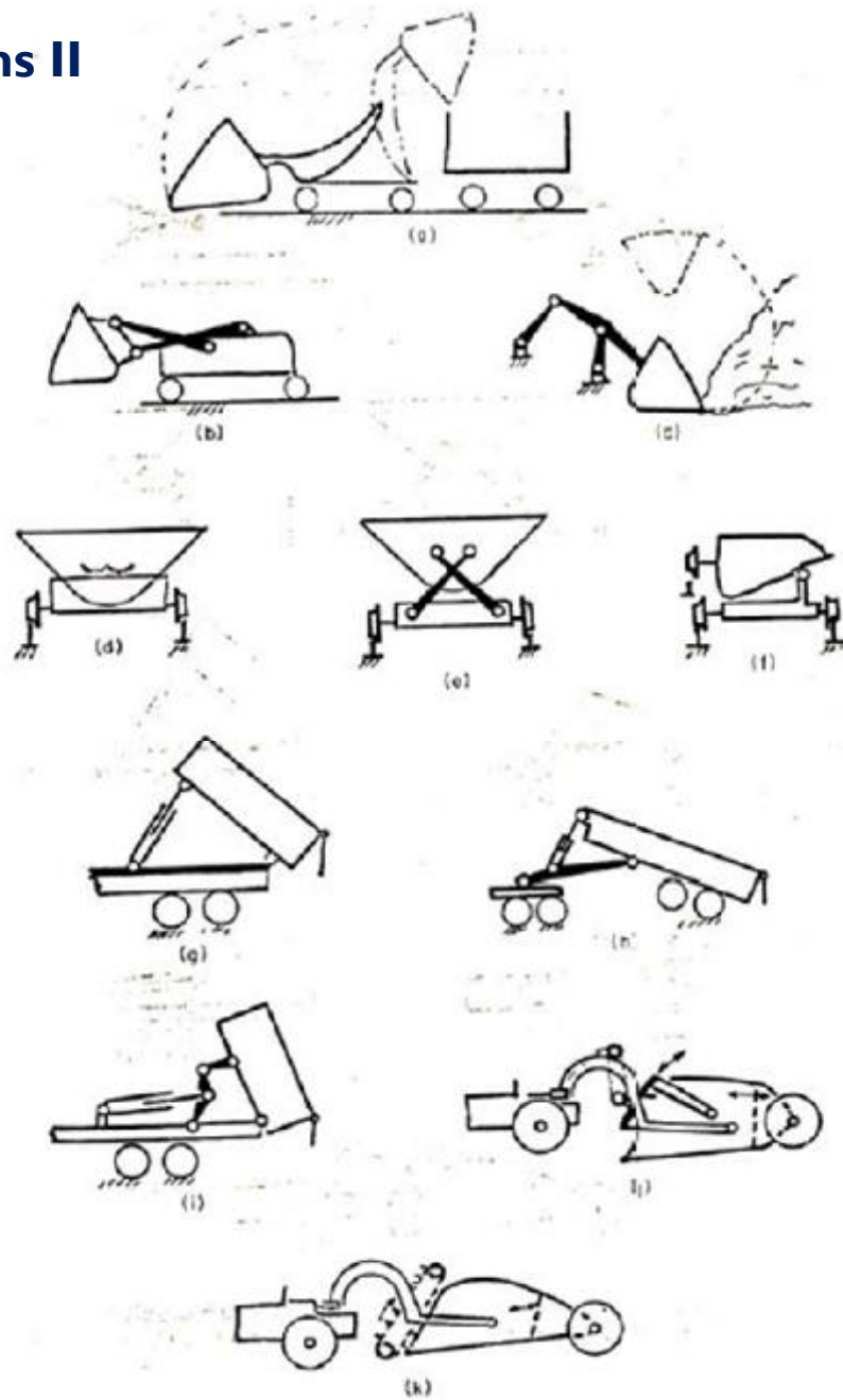
FIG. 39-23 Loading and unloading mechanisms II. (a), (b) Mucking machines; (c) scooping mechanism; (d) to (f) dumping mine cars; (g) to (i) dump trucks; (j) motor scraper; (k) elevat-
