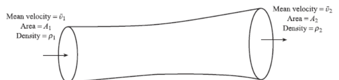
Figure 8.3 Conservation of mass flow rate in a stream tube.
