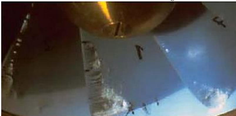
Traveling bubble cavitation in Francis turbine
