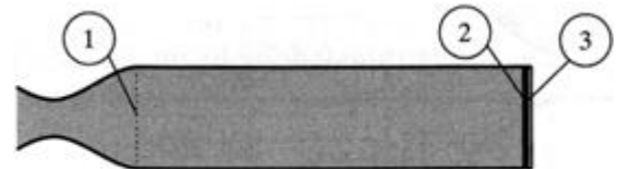
Figure 20.8b Shock at duct exit
