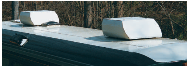
Figure 47-6 A roof-mount unit for recreational vehicles. Sometimes these are used in small stand-alone buildings. Photo by Bill Johnson
