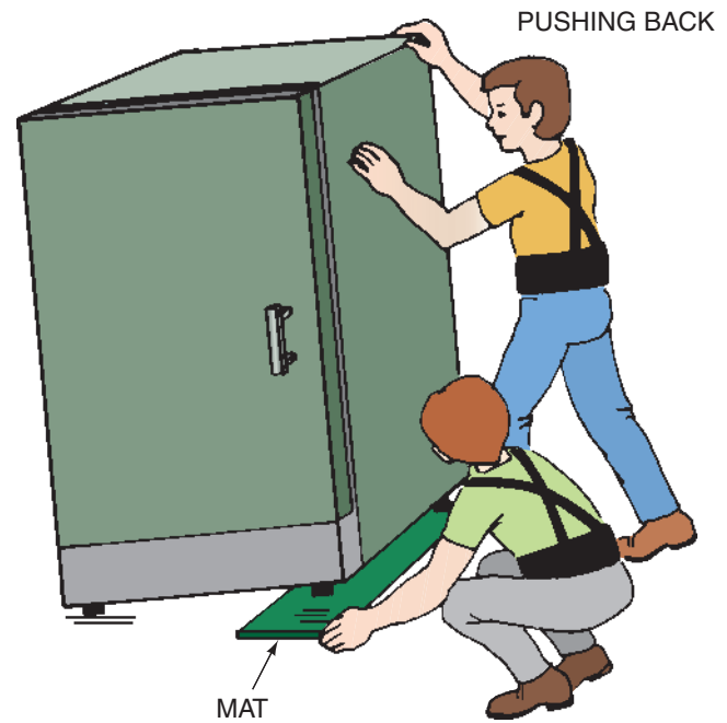
Figure 46-57 Enough room is available to tilt the freezer and place a mat under the feet.
