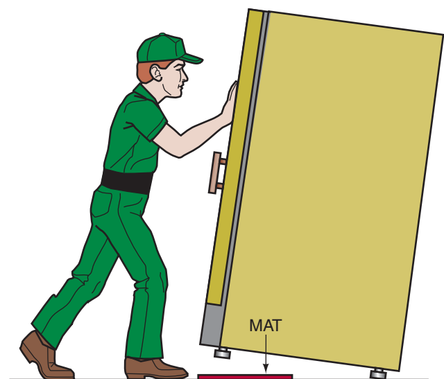
Figure 46-58 The freezer may be pulled out a few inches for the purpose of placing a mat under the feet.
