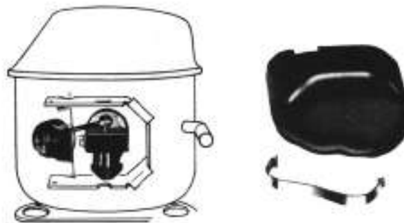
Figure(2.15)Refrigeration compressor with the thermal protector and relay assembled.
