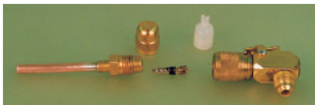
Figure 45-84 Remove the Schrader valve depressors from gage lines and use the special fitting on the right to depress the valve cores. Photo by Bill Johnson
