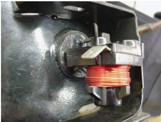
Figure 45-64 This compressor has a current relay that plugs onto the compressor terminals. Photo by John Tomczyk, Courtesy Ferris State University
