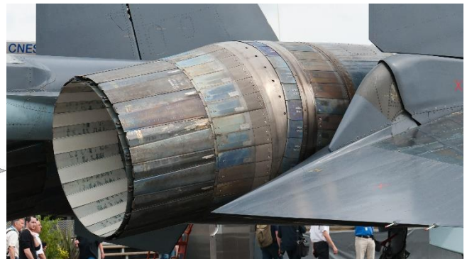
thrust vectoring by a jet engine's exhaust
