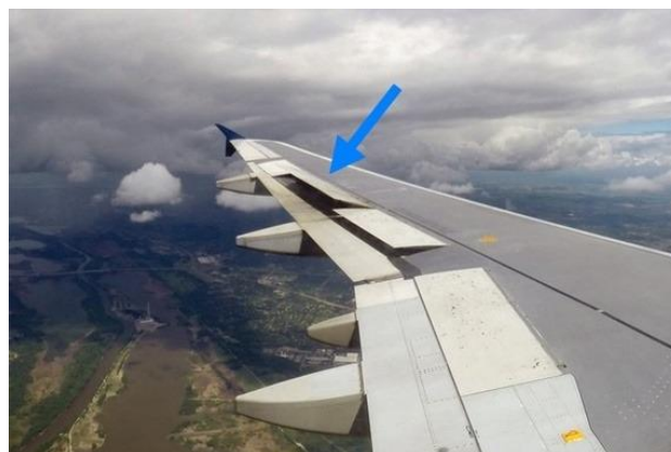
speedbrakes/spoilers mounted on the fuselage or wing
