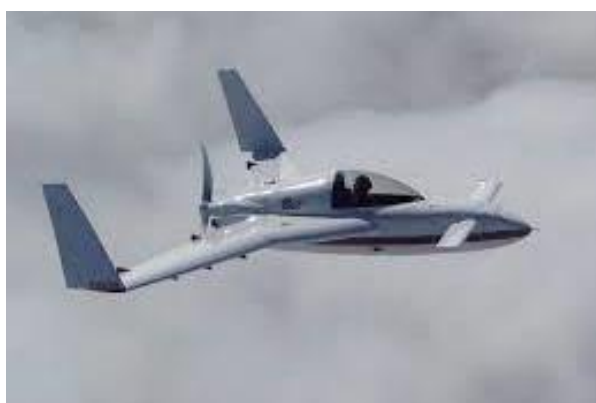
horizontal tail mounted forward of the wing (canard surface)
