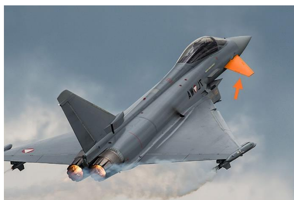
horizontal tail mounted forward of the wing (canard surface)
