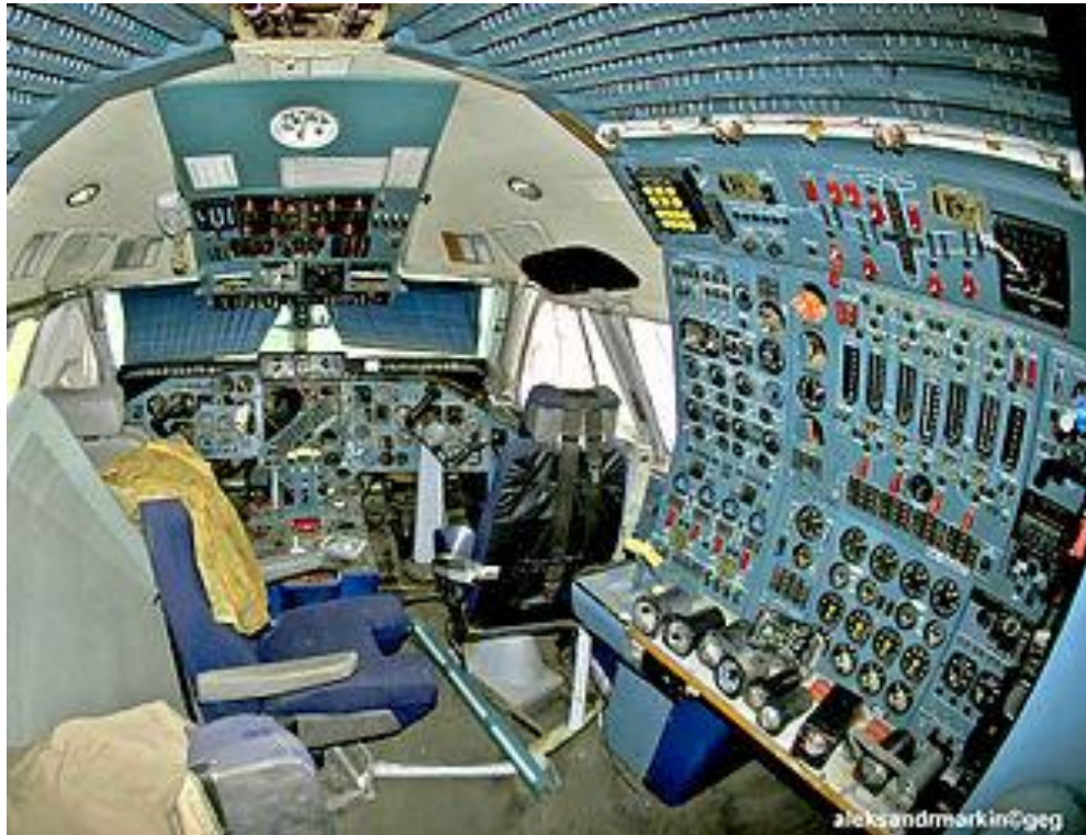
Figure 6.17 Instrument grouping at a flight engineer's station.
