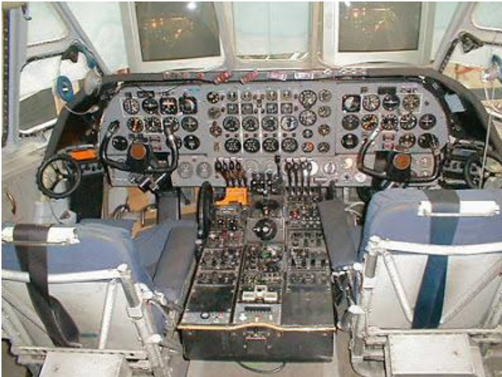
Figure 6.15 Location of instrument panels in a turbo jet airliner.
