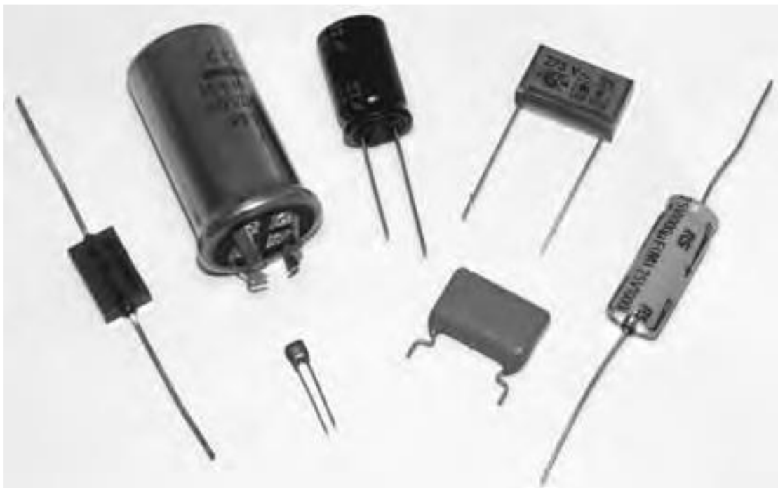
Figure 1.6 A selection of capacitors with values ranging from 12\text{ pF} to 1000\mu\text{F} and working voltages ranging from 25\text{ V} to 450\text{ V}
