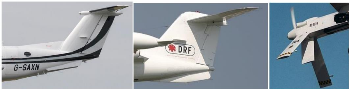
1. Beech 200 Super King Air (dorsal and ventral fin) 2. Gates Learjet 35A (ventral fin) 3. General Atomics Predator (ventral fin) (Courtesy of Jenny Coffey) (Courtesy of Antony Osborne)
