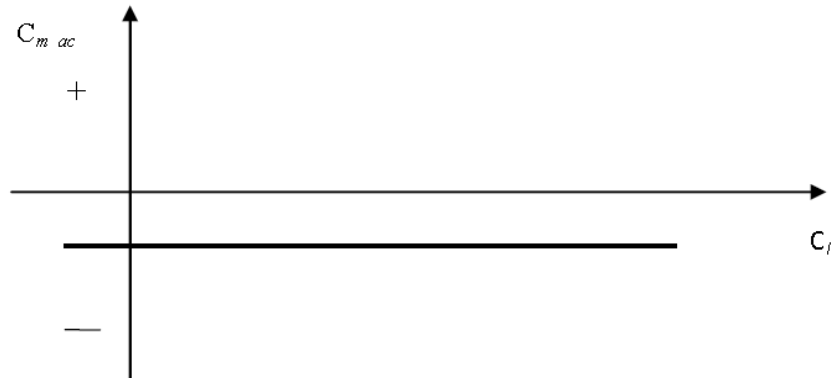
Figure 2.9: The variations of pitching moment coefficient versus lift coefficient
