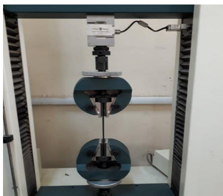
Figure 9: Tinius Olsen H50KT Tensile Machine
