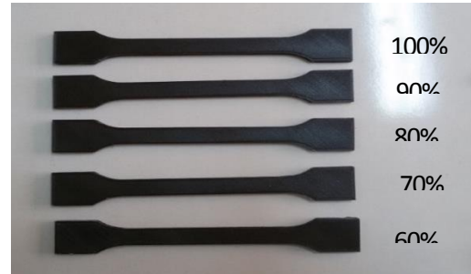
Figure 8: Carbon fiber specimens with different densities of printing
