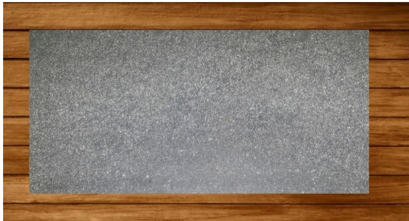
Figure (4) desiccant material coated on both sides of metal element.
