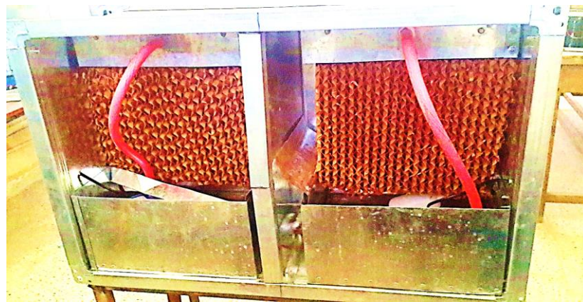
Figure (2) direct evaporative cooling after completed.
