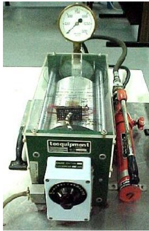
Figure 2: TecQuipment's Thick Cylinder apparatus
