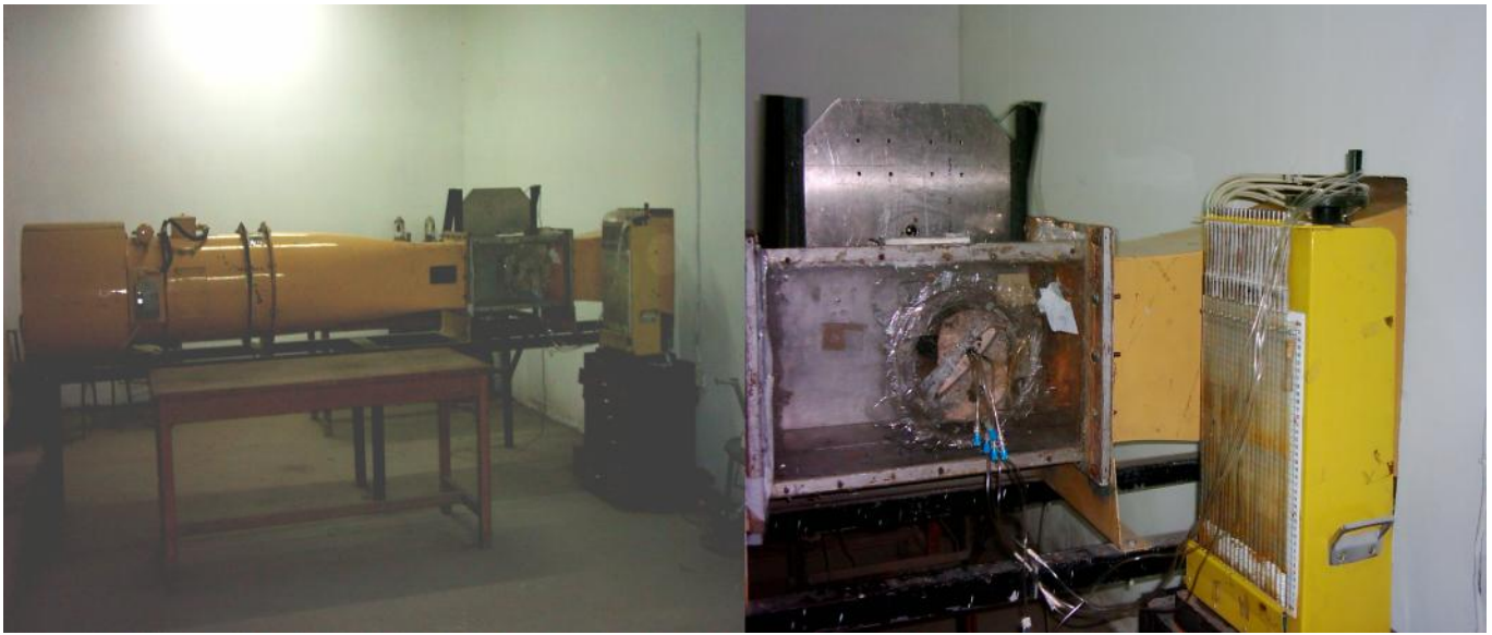
Fig. (3) Determination of C_{pu} & C_{pl} from Wind Tunnel
