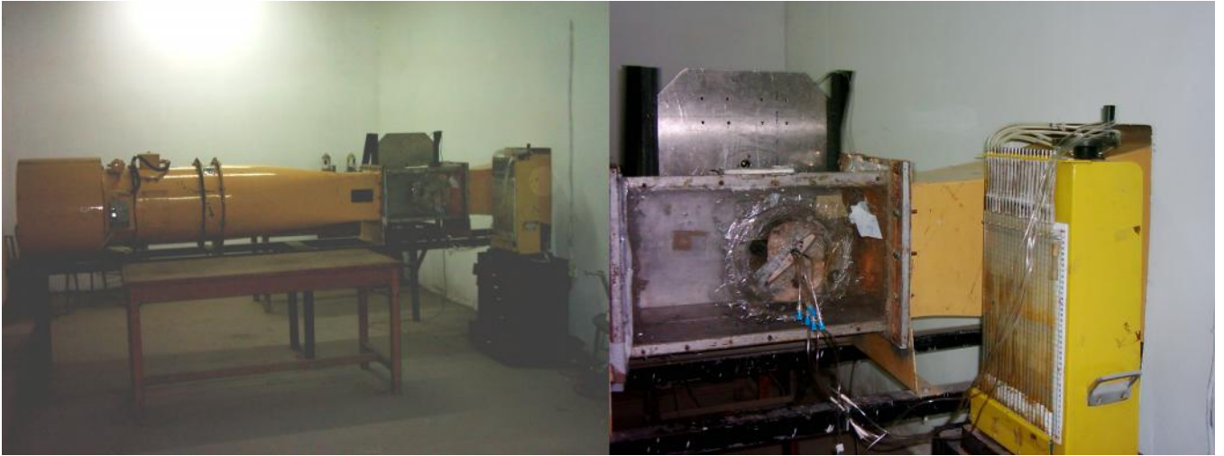
Fig. (3) Determination of C_{Pu} & C_{Pl} using Wind Tunnel
